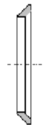
Special adapter for Satron coupling G1 Duplex adapter for installing the sensor head into the coupling (3mm depth) Product code: M1050294
