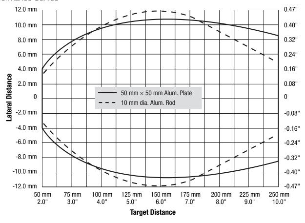
**Note:** The pattern displayed for the 50 mm  $\times$  50 mm aluminum plate is referenced to the edge of the plate. The pattern displayed for the 10 mm dia. aluminum rod is referenced to the center of the rod.
