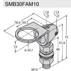
3011185 Mounting bracket, stainless steel, for M10 x 1.5 thread, thread length 30
