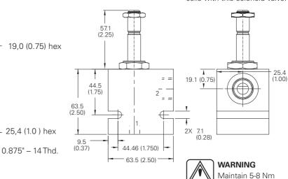
(4-6 ft lbs) maximum torque on valve tube nut.
