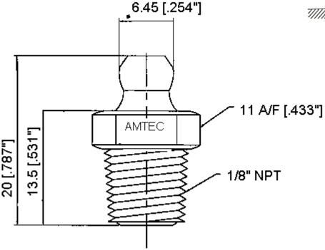
**Specially engineered one-way valve;** high pressure, heavy-duty, grease transfer fitting for use in all Amtec F-Type Hydraulic Nuts and other special lubrication applications.
