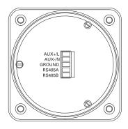
The Integra family should ideally be powered from a dedicated supply, either 100 – 250V AC or DC (85V – 280 AC absolute or 85 – 312V DC absolute) or 12-48V DC (10.2 – 60V DC absolute). However, all Integra devices may be powered from a signal source, if in the working range of the chosen auxiliary supply.
