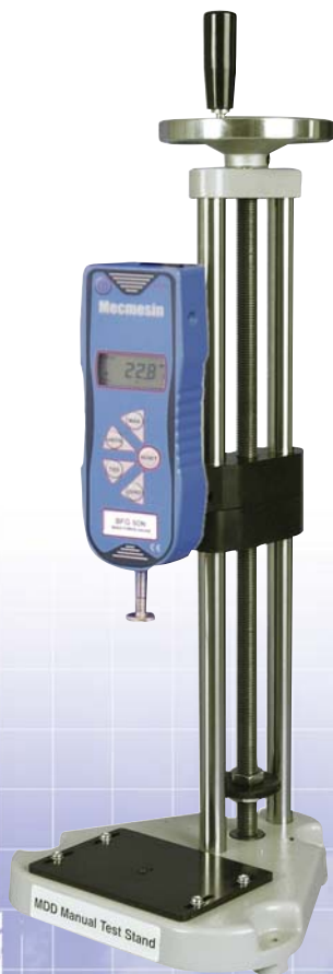
BFG shown mounted to the MDD manual test stand
