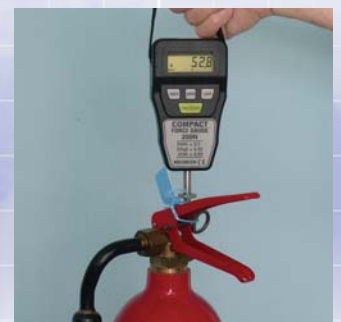
Testing fire extinguisher
